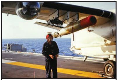
S2E Tracker anti-submarine aircraft loaded with a MK 44 homing torpedo off Hawaii for RIMPAC 72 exercise. Our aircraft carried MK 44 torpedoes on wing stations and MK 46 torpedoes in the torpedo bay (like a bomb bay) inside the aircraft.
